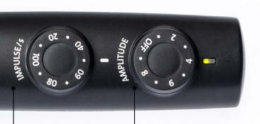
The Impulse/s setting determines the pulse frequency from 10 to 100 Hz according to the indication and recommendations in the Therapy Guide.
